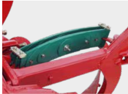
Double spring package with 14 leaves (1400 kp)
