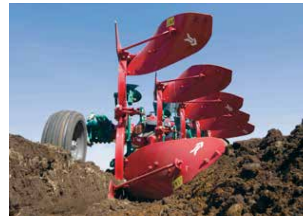
furrow profile body No. 28 working depth: 26 cm, bottom: 30 cm, width 73 cm
